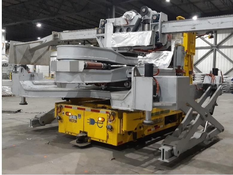
Figure 2. ARFT transported by EPIQ AGV hauler
